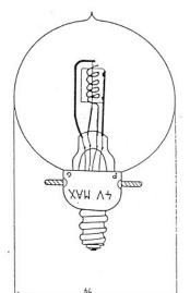
Péri then succeeded in 1915 in making a tube with movable electrodes! This permitted the behaviour of a tube to be studied experimentally, which was very useful for the theory was then by far incomplete.
