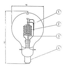
Before we come to the TM tube we know, a number of stages were gone through. First, one began with the copying of the de Forest audion, as shown in the figure above; (vertical structure, M-form filament). It turned out to be too delicate and too unstable. Then one made a model based on the "pliotron" of Langmuir. This was of
